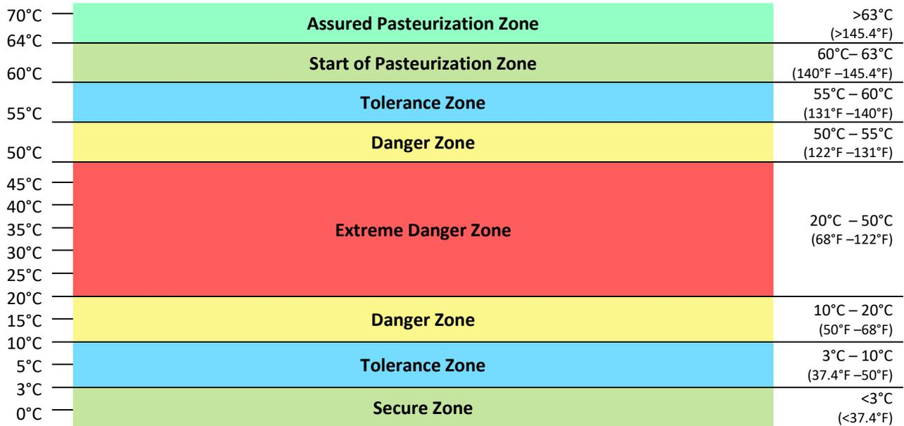
**Figure 1 – Sous vide temperature safety zones**
