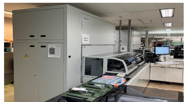
Image 2: Two refrigerated storage units connected to the line which hold a combined 30,000 samples.
