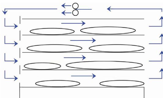
Horizontal flow is used for products that need to be placed on screened trays (ie. fish fillets)
