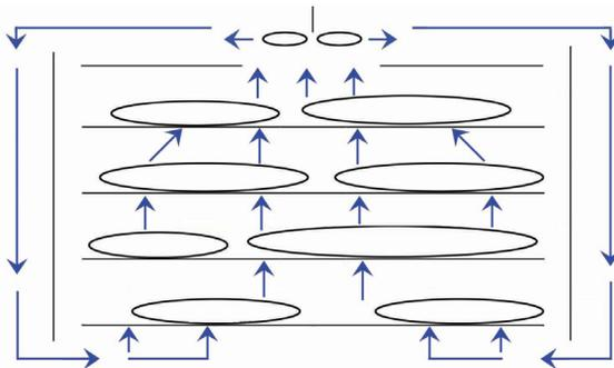
Vertical flow is used for products that are hung from rails (whole fish)
