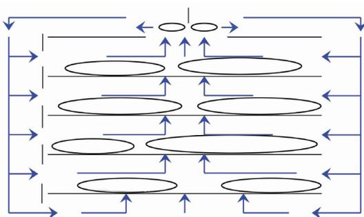
Modified systems (both horizontal and vertical flow) have uneven patterns because more air is forced through the top racks than the bottom. As a result, if the products are not left in the system long enough there may be not be an effective amount of smoking and drying.
