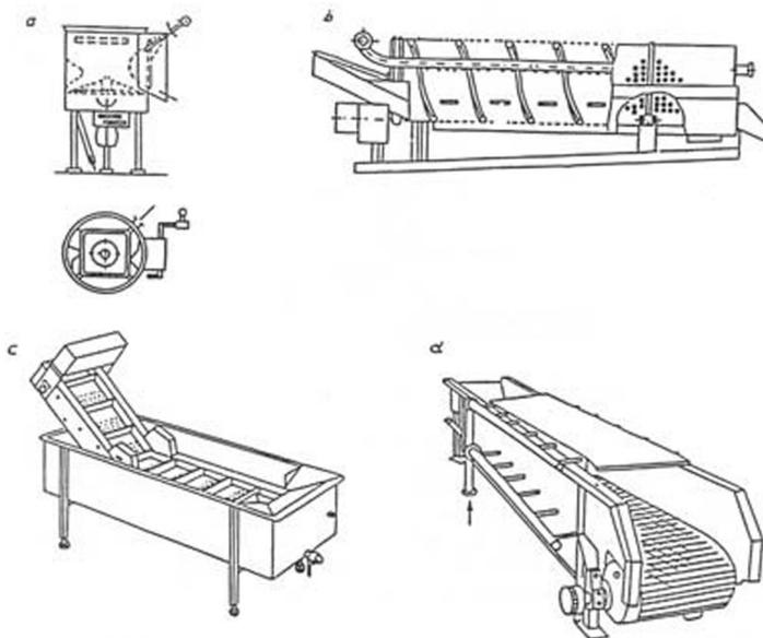
**Figure 3.10** a. Vertical-axis drum washer
