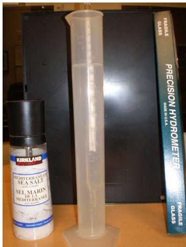
To read a salometer, place it in a see-through container which holds a sample of the solution being measured. The depth at which it floats measures the brine concentration. Readings
