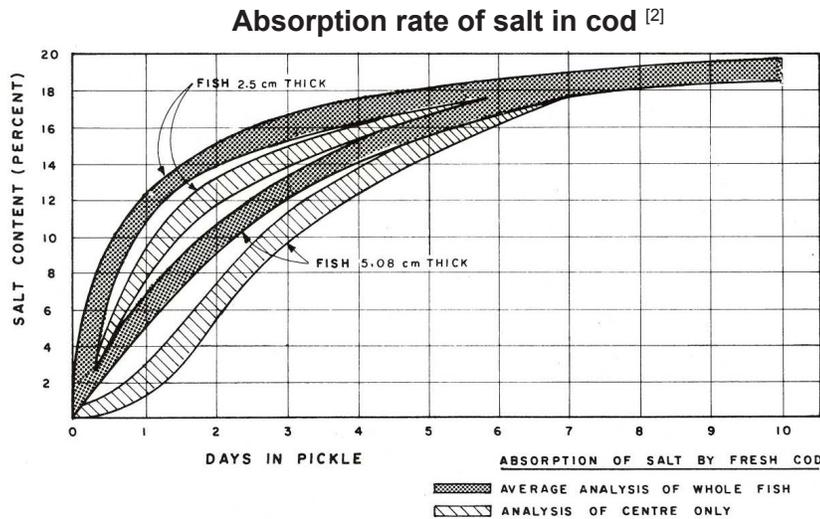
FIGURE 11.5. Absorption rate of salt by fresh cod during brine salting (Source: Beatty and Fougere, 1957).
