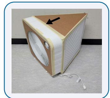
Double box fan filter. Align the arrows on the filter with the air flow of the fan.
