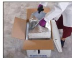
*The Softbox thermal shipping container has compartments that allow dry ice to be distributed on all sides of the box. They are only accessible after removing the dry ice pod.*
