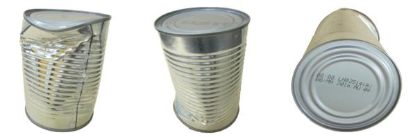
These cans of food were received on Aug 14, 2014. Although the photo at right shows the best before date is Aug 4, 2016, the dents in both these cans are too severe to accept. Dents that may affect seams or place pinholes in the can destroy the can integrity, and may allow intrusion of bacteria.
