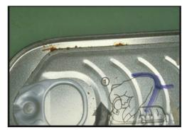
Damage to score-line (rusting from leakage)
