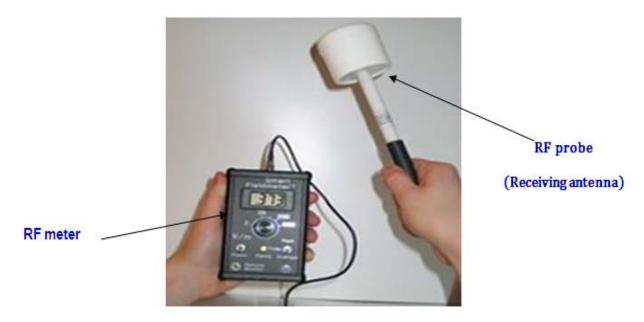
Figure 4.2 Portable RF survey meter
