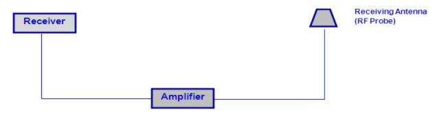
Figure 4.1 Schematic representation of a basic RF-measuring meter
