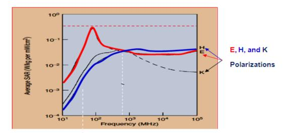
Figure 4.5 Calculated whole-body average SAR (W/Kg per mW/cm<sup>2</sup>) versus frequency for models of the average man for three standard polarizations
