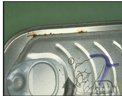
Damage to score-line (rusting from leakage)
