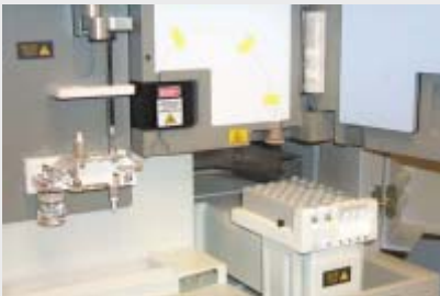
ABI 310 DNA Sequencer used for species identification
